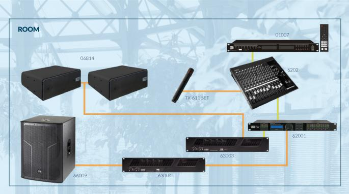
The example above is an example of a professional installation for a party room with 2 stages, one for subwoofers -66009- and another one for the line arrays -06814- and the mixing console with microphone and music source.
